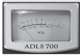
**VU Meter:** The analog VU meter displays the ADL 700's output level. When the Meter – GR switch is enabled, the VU meter will show the amount of gain reduction being applied by the compressor.
